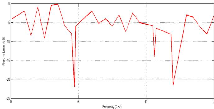
Fig. 5. Return loss versus frequency (measured)
