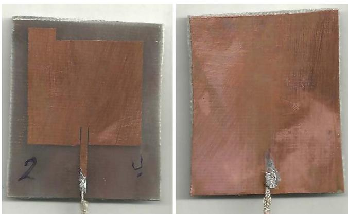
Fig. 1. A fabricated rectangular patch antenna with a stub
