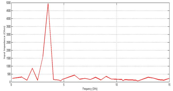
Fig. 7. Input impedance versus frequency (measured)
