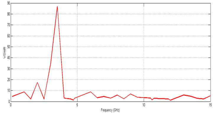
Fig. 6. VSWR versus frequency (measured)
