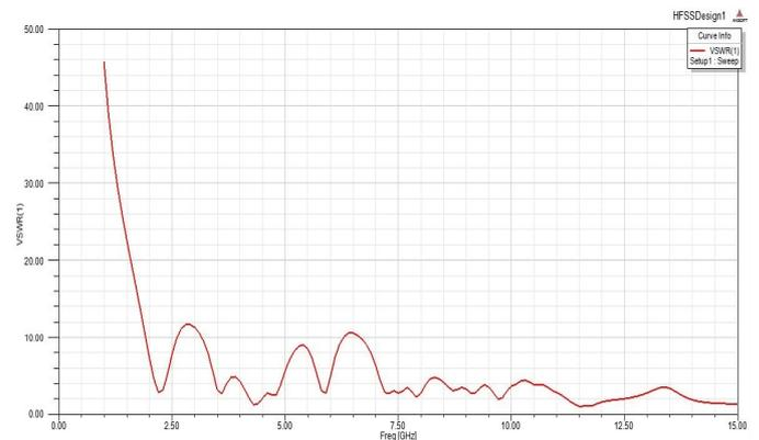
Fig. 3. VSWR versus frequency (simulated)
