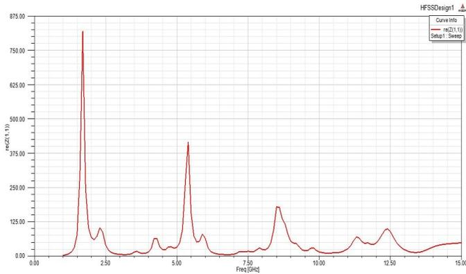
Fig. 4. Input impedance versus frequency (simulated)
